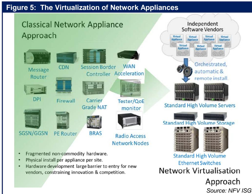
The approach that the NFV ISG is taking is that the virtualization of network functionality is applicable to any data plane packet processing and control plane function in both fixed and mobile networks. As shown in **Figure 5**, examples of these functions include:
