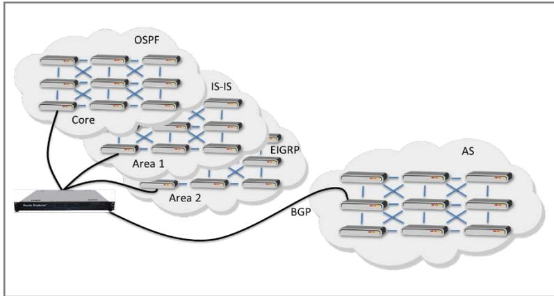
Using Packet Design’s patented technology, the Route Explorer system participates passively in the network and subscribes to all routing announcements. It records these messages and uses them to calculate and maintain a real-time model of how the network forwards traffic. It maintains the changes in a time-indexed data base so that the network forwarding model and events for a time period in the past can be retrieved,
