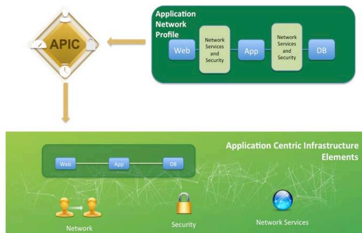
**Figure 10: Application Network Profiles are used by the APIC which pushes the required Policy to the Fabric**
